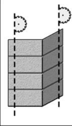
Corners can be cut to fit the remaining space at the end of the row of *Stucco Clad* panels.
