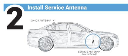
Install **Service Antenna** in the cab, towards the front, where coverage is needed. Ideally, there should be substantial material, like the metal of the roof, between the **Donor** and **Service Antennas**, to improve isolation.
