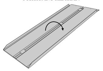
Carry the ramp to the required area using the carry handle. Fold out the ramp so it is as shown in the diagram above.
