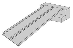
Position the ramp so the top of the ramp is higher (the top of the ramp has two holes drilled).
