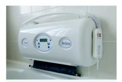
With the belt slackened, free the end secured to the floor bracket. Next **REMOVE THE BELT SLEEVE** and then press the UP button and the belt will retract. Ensure that the belt is level and square as it feeds back into the bath lift unit. Leave about 75mm (3") of the belt outside the unit so that it is easy to access for the next use. Allow the belt sleeve to dry naturally to avoid crinkling
