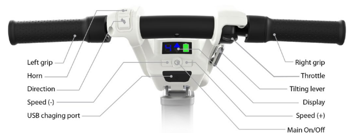
Figure 27 Driving Console overview
