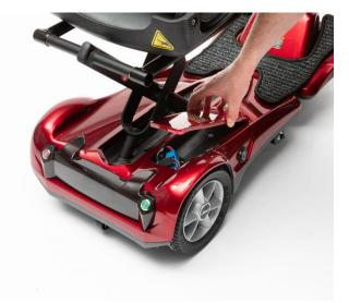
5. Turn the tiller adjustment knob anticlockwise to loosen. Pull up the tiller to the desired height. Turn the knob clockwise to secure.
