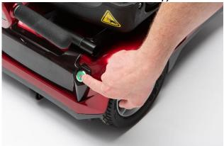
4. Push the cables in the small void behind the battery. Install the battery cover over the battery compartment (as shown above).
