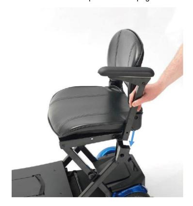
9. Secure the armrest by screwing the threaded knob into the hole (arrowed).
