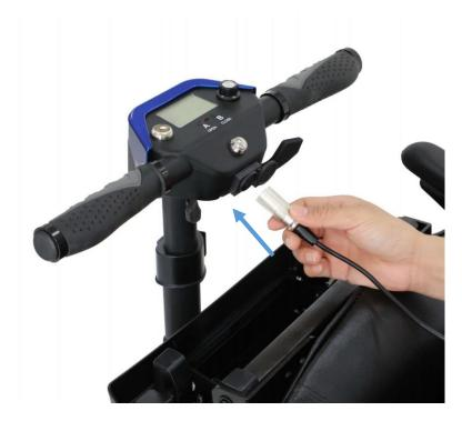
3. Insert the key into the ignition (as shown below) and switch the scooter on. Then press the button marked "A - Open" for 1 second. The scooter will then slowly beep and unfold. For safety, the unfold process will stop halfway. Press the button again to fully unfold the scooter. When fully unfolded the scooter will emit three quick beeps. Switch off the scooter.
