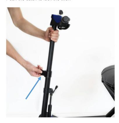
7. Adjust the tiller angle by pressing the lever (arrowed) whilst pulling or pushing the tiller to the correct angle. Release the lever to lock the tiller in position.
