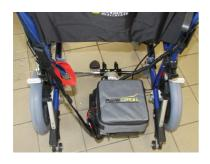
Slide the telescopic section out until the other end of the bar locates fully in the hole of the bracket on the opposite side of the wheelchair.
