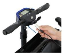
3. Insert the key into the ignition (as shown below) and switch the scooter on. Then press button on the tiller dash marked 'A-OPEN'. The scooter will then slowly beep and unfold. For safety, the unfold process will stop halfway. Press the button again to fully unfold the scooter. When fully unfolded the scooter will emit three quick beeps.
