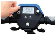
Step 2: Press the A-Open button on the control panel for 5 seconds and then release it. The buzzer will sound continuously, indicating that the control is ready to pair to the key fob.
