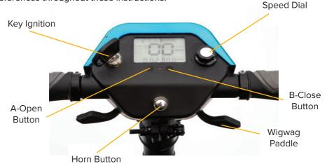
The scooter features an LCD display (right).
