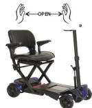
Note: You can fold or unfold the scooter manually by releasing the red manual fold release lever. If this is performed, then the opposite action should also be performed manually to reset. Failure to do so will not damage the scooter, but the autofold function may not work until the folding mechanism is manually reset. For this reason, it is recommended the manual operation is performed in emergency only.
