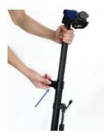
6. Pull on the catch (arrowed left) on the tiller to unlock. Then pull up the tiller until it is set at the correct height for the user. Push the catch to lock the tiller.
