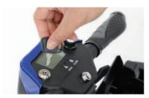
4. Pull up the strap on the battery so that the plastic insulation strip can be removed, then refit the battery pack as shown.
