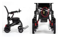
4. Put freewheel levers into 'Electric' mode by pushing forward both levers towards the chair. Press in the latch and extend the anti-tip wheel backwards, on both sides of the powerchair.
