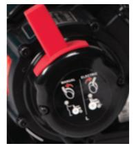
Figure 1 – Electric / Manual mode switch
