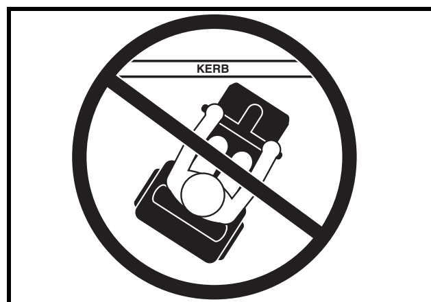
Figure 3A. Incorrect Kerb Approach
