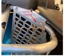
NOTE: Depending on the tools you have on hand it may be easier to complete Step 5B with the mounting bracket off the snowmobile before you complete Step 4 & 5A. I find it easier to place the rivets this way if you have a air rivet gun. If you have a manual hand rivet gun follow the installation steps in the order below.
