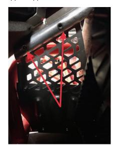
**Step 2:** Remove exhaust side panel and push dart connector circled once side panel is removed.
