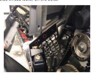
\*Note: It is also highly recommended to drill a 3/16" hole in the mounting tube using the pilot holes highlighted in the above picture as a guide and place the additional 3/16" flange head rivets included in the highlighted locations. This reduce stress on the factory mounting inserts and give additional level of protection against pull out of the factory mounting inserts.
