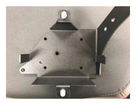
**Step 3:** Locate the (2) factory mounting locations on the upper support tube inside the foot well.
