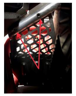
**Step 4:** Install Battery and Cover with supplied ¼-20 hex head locknuts. The top mounting flange may need to be bent down slightly to make the studs line up with the holes in the cover. This is normal because it was designed to slightly pinch the top of the battery to help it hold in its location.
