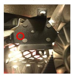
\*Note: Also recommended is to drill 3/16" hole in factory tube using highlighted hole above as a guide and place a 3/16" rivet in that location.
