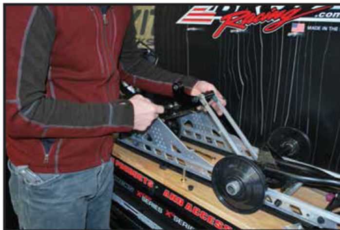
ASSEMBLE TO STOCK SHOCK GUIDE RODS USING STOCK HARDWARE.
