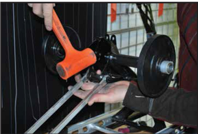
USE SUPPLIED HARDWARE TO INSTALL ARSFX UPPER LINKAGE BRACKET.
