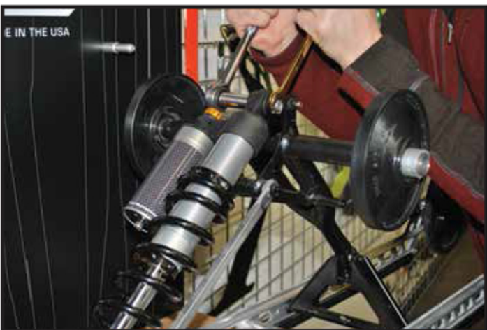
INSTALL EXIT SERIES REAR SHOCK USING STOCK HARDWARE AND TIGHTEN.
