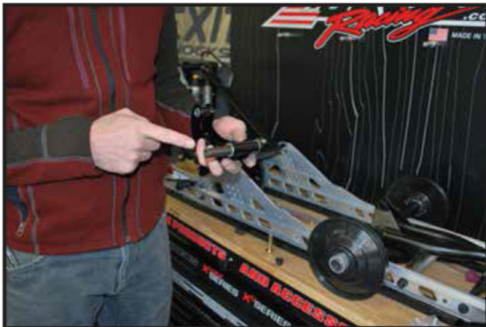
INSTALL STOCK PIN INTO ARSFX LOWER LINKAGE BRACKET.
