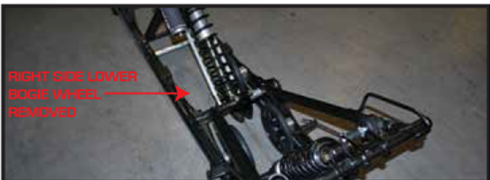
INSTALL EXIT SERIES REAR SHOCK USING STOCK HARDWARE AND TIGHTEN.
