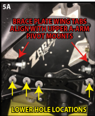
5A. ALIGN EXTERNAL SIDE BRACE PLATE BY INSTALLING UPPER A-ARM BOLTS THROUGH BRACE PLATE WING TABS. DRILL (4) LOWER HOLE LOCATIONS AND RIVET IN PLACE USING (4) 1/2" RIVETS (SEE YELLOW ARROWS).
