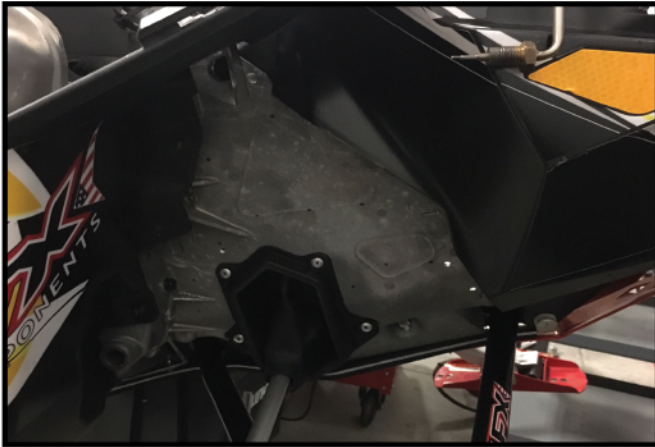
1. REMOVE HOOD, PIPE, SKI SHOCKS AND UPPER A-ARMS.
