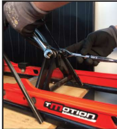
5. REMOVE REAR SCISSOR ARM BOLT. KEEP STOCK WASHER AND NUT TO BE REUSED IN STEP 5.
