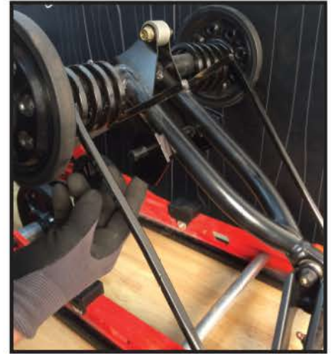
3. INSTALL NEW BILLET TORSION SPRING BLOCKS. REFER TO STEP 4 IF RUNNING OUR T-MOTION COIL OVER CONVERSION REAR SHOCK.
