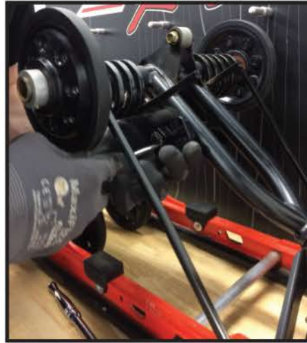
2. REMOVE C-CLIPS FROM TORSION SPRING PRELOAD BLOCKS.
