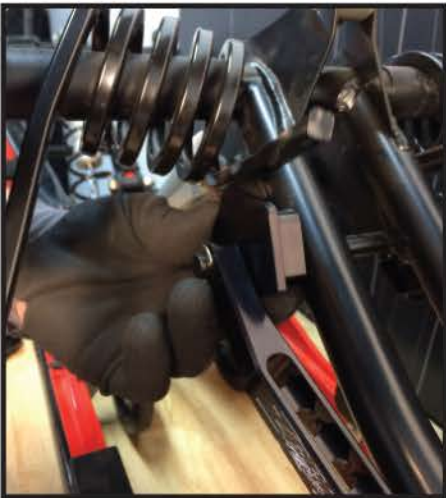
6. POSITION BILLET TORSION SPRING BLOCKS AND BILLET LINK RODS TO REAR SWING ARM ASSEMBLY AND ATTACH STOCK C-CLIPS.
