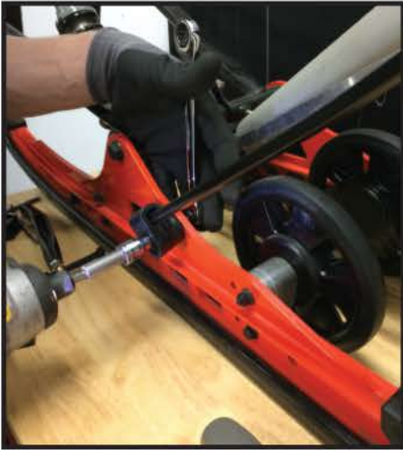
1. REMOVE TORSION SPRING FROM RAIL SPRING RETAINER.
