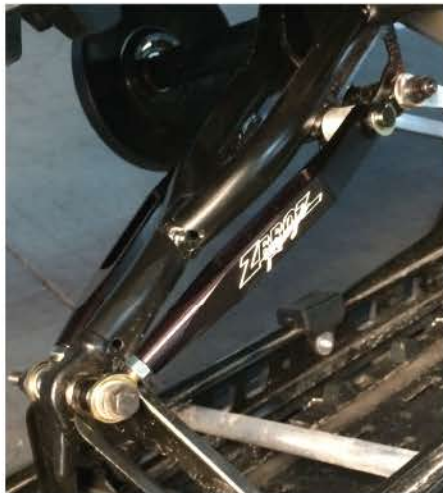
4. IF YOU ARE RUNNING OUR T-MOTION COIL OVER CONVERSION REAR SHOCK, YOU WILL USE SUPPLIED SPACERS INSTEAD OF BILLET TORSION SPRING BLOCKS.
