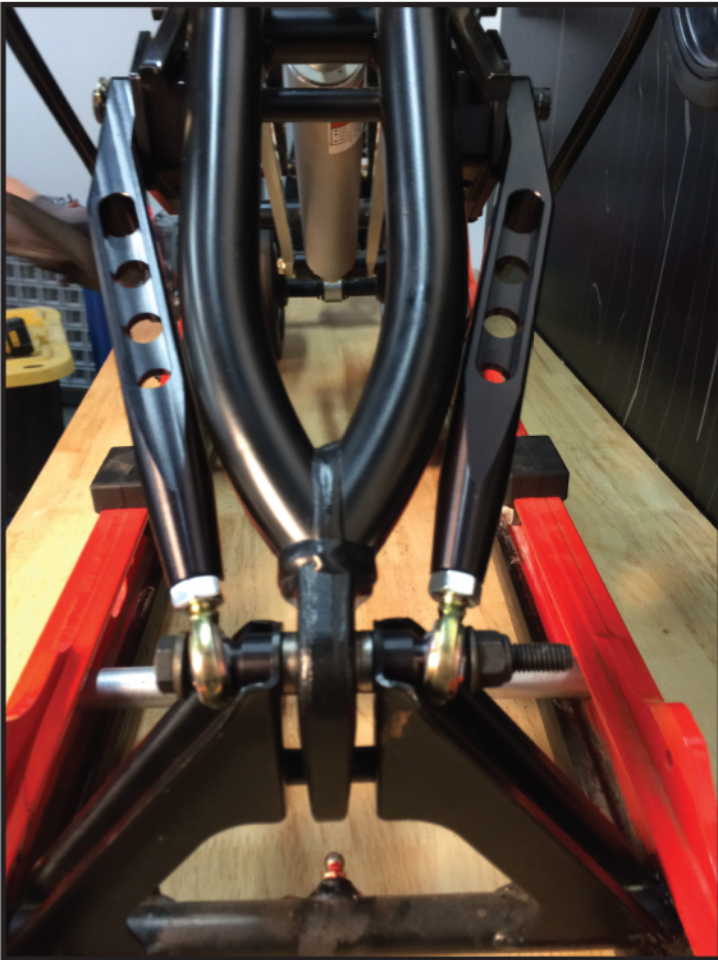
7. ADJUST HEIM JOINTS TO ALIGN BILLET LINK RODS TO REAR SCISSOR ARM BOLT HOLE ASSEMBLY AND TIGHTEN HEIM JOINT JAM NUTS. TIGHTEN REAR SCISSOR ARM BOLT.
