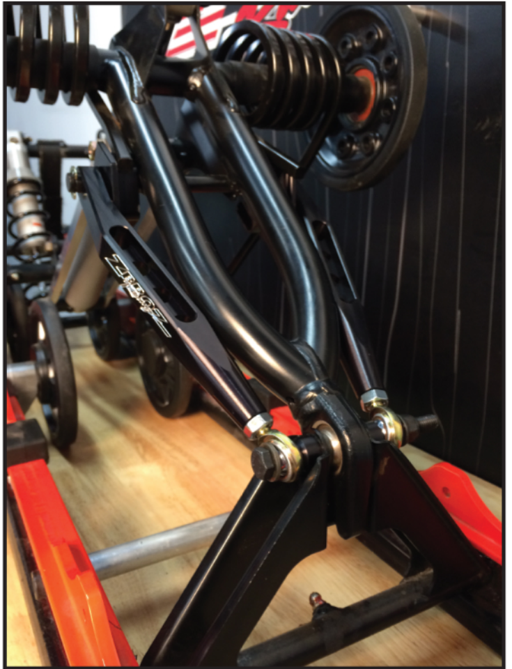
7. ADJUST HEIM JOINTS TO ALIGN BILLET LINK RODS TO REAR SCISSOR ARM BOLT HOLE ASSEMBLY AND TIGHTEN HEIM JOINT JAM NUTS. TIGHTEN REAR SCISSOR ARM BOLT.
