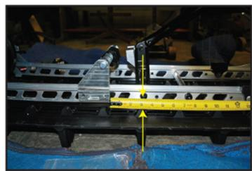
2. POSITION K.I.S.S. COUPLER ASSEMBLY 3 1/8" BACK FROM BOTTOM SCISSOR ARM BOLT MOUNT LOCATION. TIGHTEN TOP K.I.S.S. COUPLER BOLTS TO HOLD IN PLACE.
