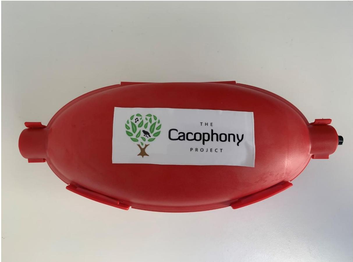
The Bird Monitor comes in a weatherproof box and should be mounded ideally where it is shaded, so it does not get too hot and where it has some shelter from the rain. There is enough room in the box for the phone to be plugged into an extension cord of this is going to be run off mains power.
