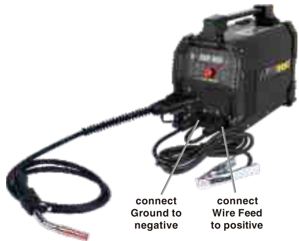
DCEP Solid Core (Gas Shielded) Polarity Setup
