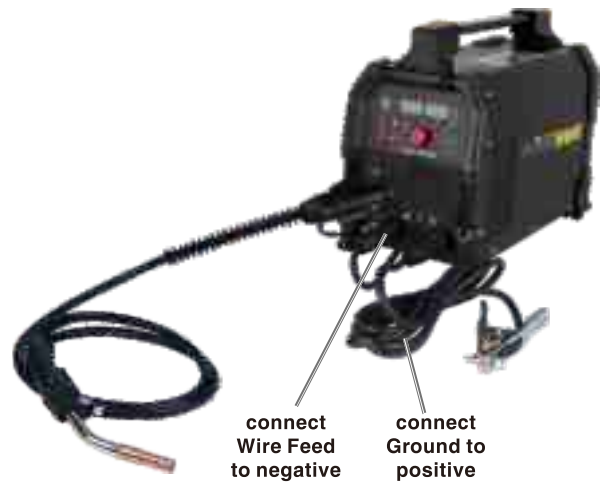
DCEN Flux-Cored (Gasless) Polarity Setup
