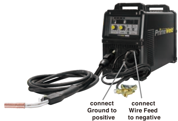
DCEN Flux-Cored (Gasless) Polarity Setup
