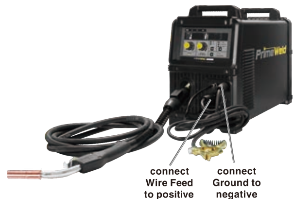
DCEP Solid Core (Gas Shielded) Polarity Setup
