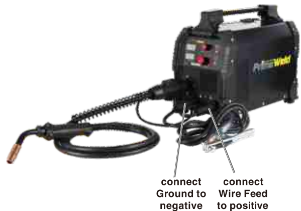
DCEP Solid Core (Gas Shielded) Polarity Setup
