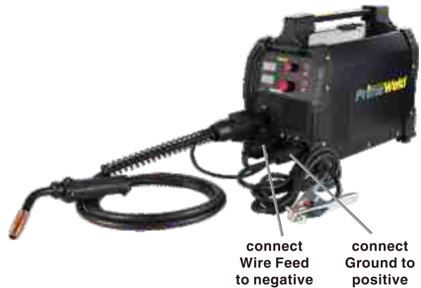
DCEN Flux-Cored (Gasless) Polarity Setup
