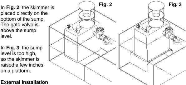
If your system does not allow for an in-sump installation, it is easy to install your skimmer outside of the sump. If vertical clearance isn't an issue, the best solution is to raise the entire skimmer on a platform so that the gate valve will clear the sump wall. If you don't have the clearance to raise the skimmer, you can install a 1" bulkhead through the side of the sump wall and directly connect the skimmer to the sump.
