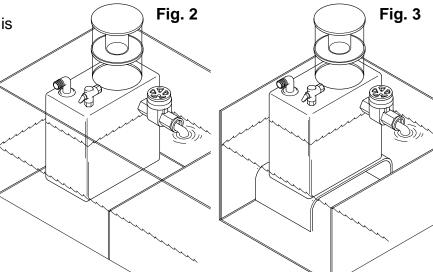
If your system does not allow for an in-sump installation, it is easy to install your skimmer outside of the sump. If vertical clearance isn't an issue, the best solution is to raise the entire skimmer on a platform so that the gate valve will clear the sump wall. If you don't have the clearance to raise the skimmer, you can install a 2" bulkhead through the side of the sump wall and directly connect the skimmer to the sump.
