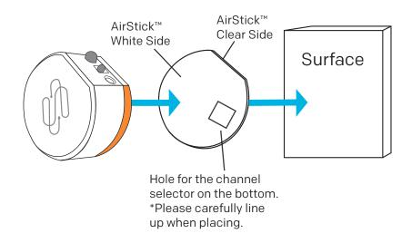
To keep the BlastIR Wireless in one place, we have included Airstick<sup>M</sup> and  $3\text{M}^{\text{M}}$  adhesive. Airstick<sup>M</sup> is used as pictured above and it is designed to be reusable and leave no residue. The  $3\text{M}^{\text{M}}$  adhesive is used the same way and is used for a more permanent placement.
