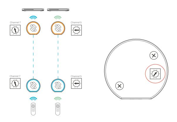
BlastIR Wireless Receivers will only communicate with the BlastIR Wireless Emitters that are set to the same zone. The Blast IR Wireless supports up to ten unique zones of communication. Setting the zone to "0" will allow communication to previous models of the BlastIR Wireless. After changing the zone, please reset the device.
