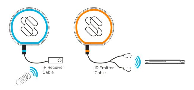
If you want to extend the reach or hide the receiver or emitter, connect the appropriate color-coded cable to the device. The blue IR receiver cable will add another receiver you can point your remote at. The orange IR emitter cable can attach to the IR "eye" of the device you wish to control.
