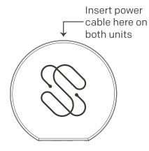
Connect each unit to power using either the included power supplies or the USB to DC cables.
