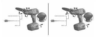
Fit the drill bit into the chuck or remove it from the chuck.
