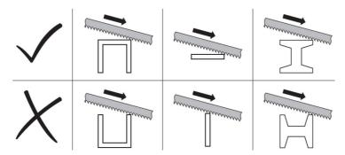
Bring the workpiece and the bandsaw into alignment.
