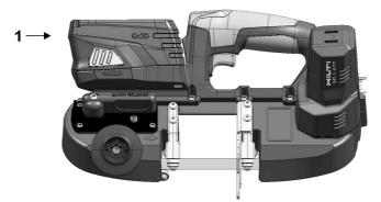
From the front, push the battery back into the product until it engages with an audible double click.
