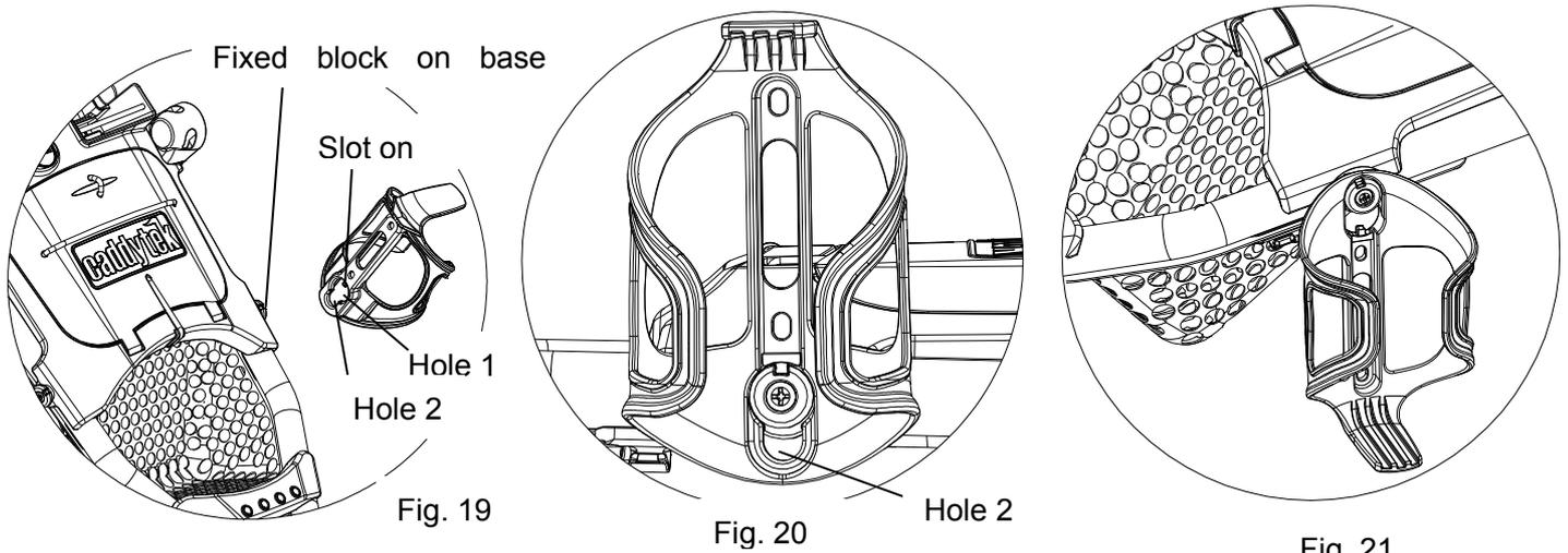
When installing the drink holder as Fig.19, align the smallest part of the slot on the holder with the fixed blocks. Then pull horizontally to fit the holder on the base as Fig.20 & 21.
