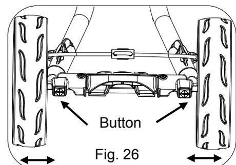
Press the button and slide the front wheel out/in ward to adjust the width between front wheels as Fig. 26, so that different sizes of golf bag can be fitted on the cart.
