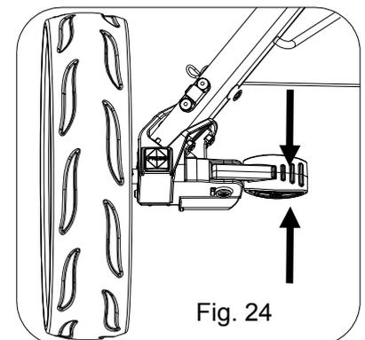
Press the foot brake to brake,
