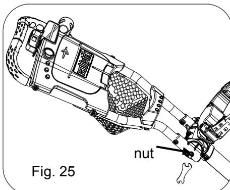
Time to time, please tight the upper connection nut with provided tool, as above Fig. 25, to prevent lose handle and prolong the life of the cart.
