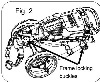
Release handle and front wheel frame locking buckles as shown above Fig.2.
