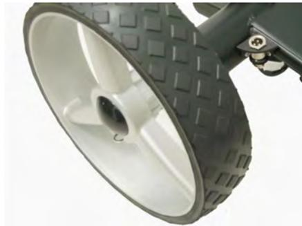
6. Insert anti tip wheel into frame and secure with pin.
