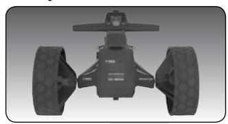
On the wheel, press the grey release button on the wheel hub. Place the wheel onto the axle. You will notice you need to match up the inner female groove on the axle and the male of the wheel. When placed in position simply release the button. You will notice you hear a "click" when the wheel is properly secured. To check that the wheel is properly in position pull on the wheel. If it is properly in position it will not slide off. Repeat for the other wheel.
