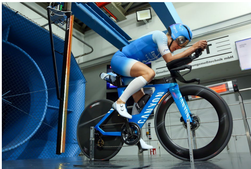
Figure 8: One athlete of the many tested with the AERO CALF Sleeves in the full-size wind tunnel.
