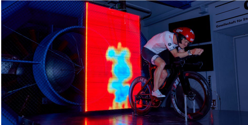
Figure 12: Aerodynamic measurements in a full-size wind tunnel on athlete without AERO CALF Sleeves. The red zone indicates no losses (100% total pressure). The darker the blue, the more the losses/aerodynamic drag.
