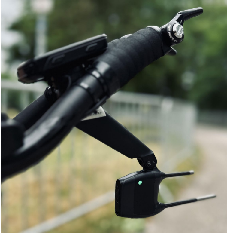
Figure 3: CDA meter for aero measurement
