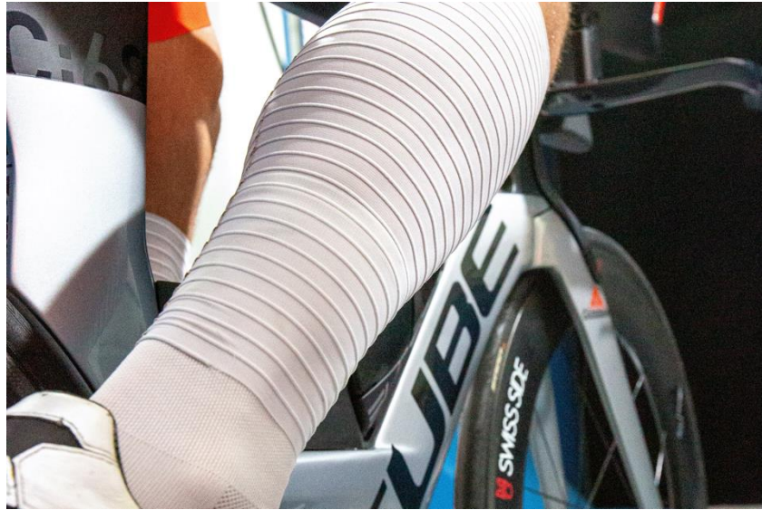
Figure 11: Fabric sample T13 in an early prototype phase in full-size wind tunnel with an athlete.
