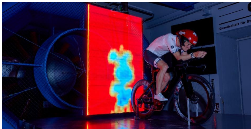
Figure 9: Aerodynamic measurements in a full-size wind tunnel on athlete without AERO CALF Sleeves. The red zone indicates no losses (100% total pressure). The darker the blue, the more the losses/aerodynamic drag.
