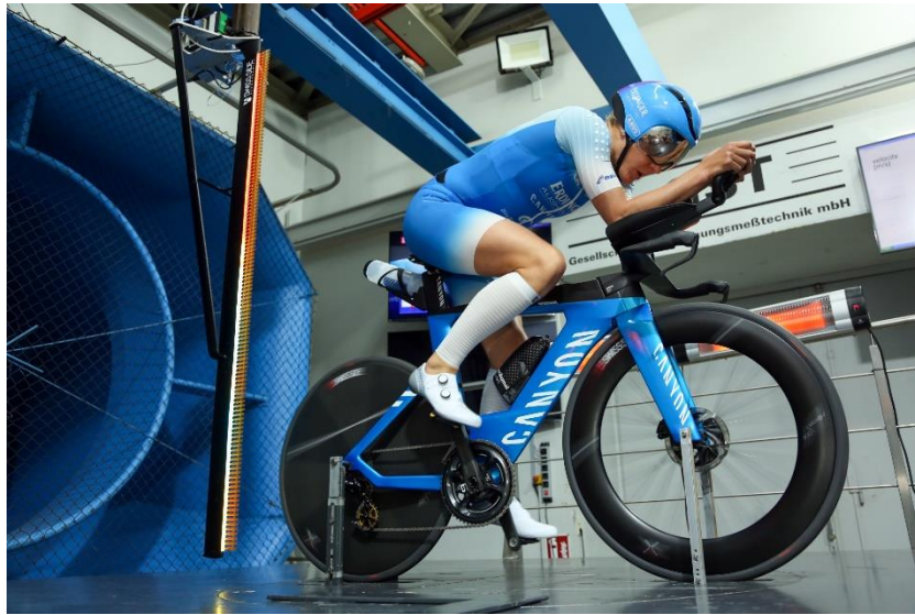
Figure 9: One athlete of the many tested with the AERO CALF Sleeves in the full-size wind tunnel.
