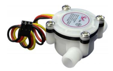
Water flow sensor consists of a plastic valve body, a water rotor, and a hall-effect sensor. When water flows through the rotor, rotor rolls. Its speed changes with different rate of flow. The hall-effect sensor outputs the corresponding pulse signal. This one is suitable to detect flow in water dispenser or coffee machine.
