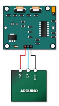
The sketch simply turns on Your Arduino LED connected to Pin 13 whenever motion is detected. Be sure to beware of and somehow handle the 1 minute initialization in whatever application you develop.
