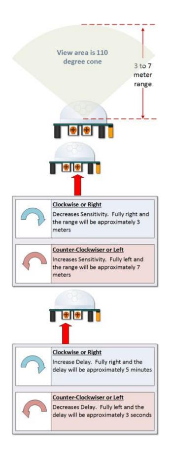
The device will detect motion inside a 110 degree cone with a range of 3 to 7 meters.
