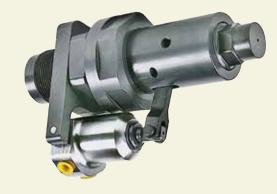
The injection orifice of the power operated nozzle can be opened without pressure loss. The nozzle is controlled by hydraulic or pneumatic actuation. The reliable shut-off system separates the melt flow at a predefined point determined by the process. The control of opening and closing is integrated into the unit and is very compact.
