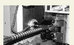
**Nitrided barrels**- We hold stocks of ready bored and honed barrels for immediate manufacture significantly reducing lead times. Sizes start at 18mm ø bore. Nitriding is conducted for the maximum time possible to create the thickest case depth.
