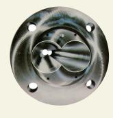
Twin Conical Barrels – similar criteria as for parallel barrels, but high throughput and specialised equipment keeps prices low when compared to original equipment from manufacturers.
