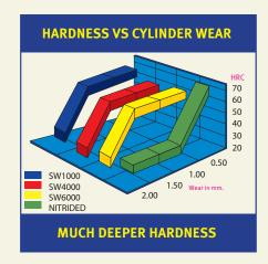
Particle Metallurgy Steels are throughhardened and wear characteristics do not degrade as the surface is eroded.
