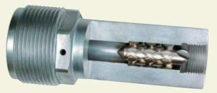
Recess is machined into nozzle in our workshop. Elements slide into nozzle recess. Standard nozzle tip is used.
