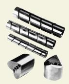
Forced radial mixing is one of the fundamental reasons for the superior performance of the ISOMIX MOTIONLESS MIX NOZZLE. Figures on the left show that outer streams 1 & 4 emerge on the inside, whereas inner streams 2 & 3 migrate to the outside. The process is repeated as material flows into a tetrahedral cross section between elements resulting in positive cross blending of any temperature and colour gradients in the polymer melt stream.
