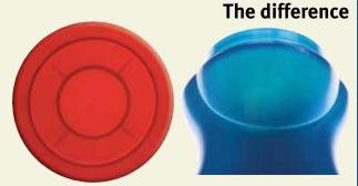
Same product, same 2% master batch additive but processed through a Nickerson Static Mixing Nozzle. The darker colour is the result of a good homogenous mix resulting in a uniform distribution of the colourant with no unplastisized particles.
