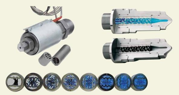
The **KSM** mixing nozzle is designed to give a high level of melt homogenisation using a wide range of materials. The mixer allows parts to be made to tighter tolerances virtually eliminating spots, streaks and clouds of colorant. Reject rates are reduced and significant savings in material are possible.
