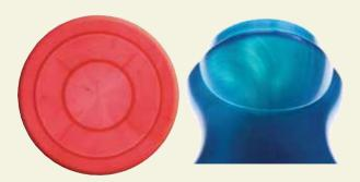
Moulding produced using a standard open nozzle with a 2% master batch additive, note the patchiness of the colour dispersion and the unplasticised particles contained within the moulding.
