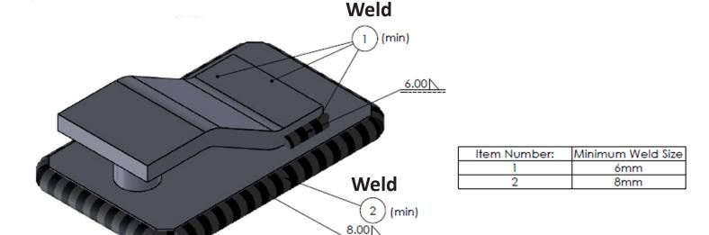
PLEASE NOTE: We recommend a minimum 8mm weld on the entire base plate, please ensure that your Chassis Specifications meet the ADR and VTA guidelines before attaching our base plate.
