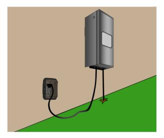
Check that both pilot lights are on inside your transformer power unit. The main pilot light for your transformer is green and right above the internal breaker. If it is not on, the transformer is not receiving power. Check if the breaker for the GFCI outlet is on. For any line voltage issues, contact a licensed electrician.
