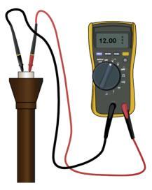
If needed, you can adjust the fixture voltage by using a higher voltage at the transformer terminal.
