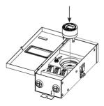
Turn the timer clockwise to the manual "ON" setting by aligning the word "ON" with the orange triangle on the left.
