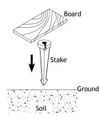
Determine the desired location for mounting the stake mount. Hammer the stake into the ground until flange of stake is flush to grade. To avoid damage to the stake, place a board on top of the stake while hammering.
