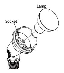
Insert the lamp with the correct wattage and type marked on the fixture label and secure into place.
