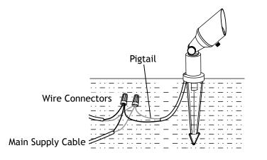
Strip both leads from the luminaire pigtail. Using two wire connectors (sold separately), connect the leads from the luminaire to the main supply cable leads.
