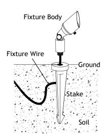
Pass the fixture wire through the center hole of the stake. Thread the fixture body onto the stake. Hand tighten until snug.
