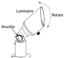
Loosen the knuckle to adjust the luminaire to your desired direction. Always tighten the knuckle once your desired direction is achieved.
