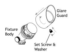
Remove the set screw and washer, rotate the glare guard counter clockwise and remove it from the fixture body.
