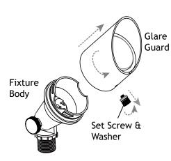
Place the glare guard back onto the fixture body and rotate it clockwise. Thread the set screw with washer back onto the glare guard.
