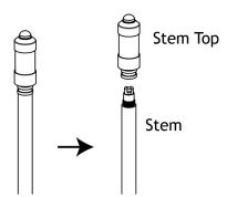
Loosen the stem top and remove it from the stem.
