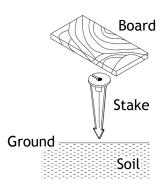
Determine the desired location for mounting the fixture. Hammer the stake into the ground until the flange of the stake is flush to grade. To avoid damage to the stake, place a board on top of the stake while hammering.
