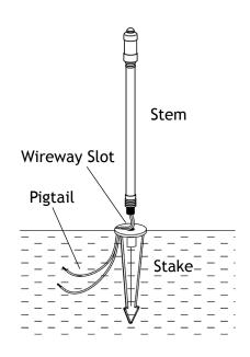
Clear away an area in the ground at the wireway slot on the top of the stake. Lay the luminaire pigtail into the wireway slot and attach the stem onto the stake. Tighten until snug.
