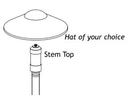
Thread the hat of your choice onto the stem top. Hand tighten until snug.
