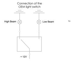
Connection for m.unit Disconnect ALL switch cables and connect as shown:
