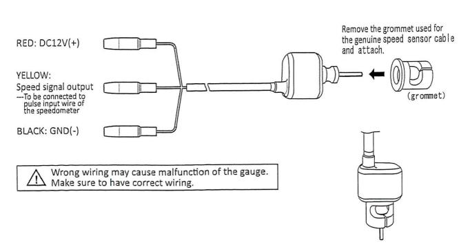
Replace the genuine speed sensor cable with this converter.
