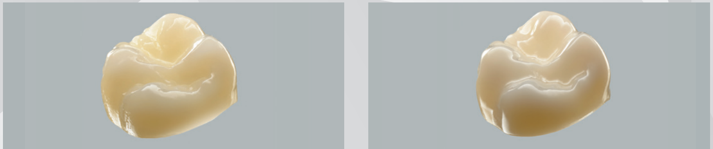
Backlight image of molar crown made of 3M™ Lava™ Esthetic Zirconia (left) compared to conventional high translucency zirconia (right). Source: 3M Oral Care internal data.
