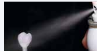
Spray the IPS e.max CAD Crystall./Glaze Spray on the unfired Shades and Stains.
