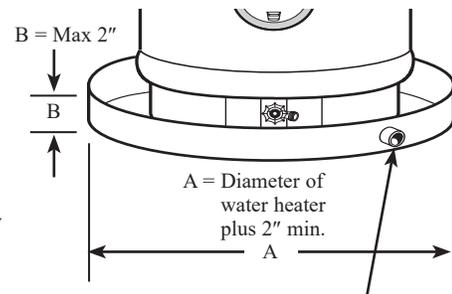
To open drain, this line should be at least 3/4" ID and pitched for proper drainage.
