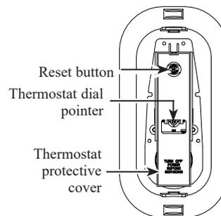
The illustration at the left shows the temperature adjustment dial used for setting the water temperature.
