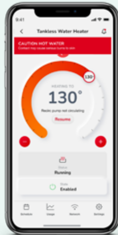
ALERTS, NOTIFICATIONS AND ERROR CODE SETTINGS Includes maintenance reminders and a scalding alert for set points above 120F.
