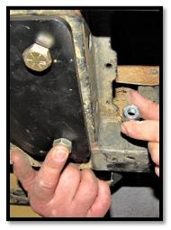
6. Using the three holes at the other side of the plate as a guide. Drill through them into the frame with a 5/16 drill bit.
