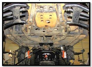
4. Starting on the PASSENGER SIDE. Place the frame mounting plate 111U-R to the fitted section of the frame.
