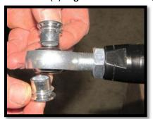
18. Slide a **12mm flat washer** onto a **½"** x **2-3/4" bolt.** Insert it though the tabs and heim. Secure it with a **12mm flat washer** and **1/2" lock nut**. Torque the nut to 110lb-ft. Repeat to other side.
