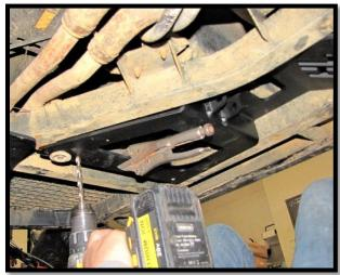
7. Slide a **5/16**" **flat washer** onto (3) **5/16**" **x 1**" **bolts** to connect the plate to the frame. Loosely secure them with **5/16**" **flat washers** and **5/16**" **lock nuts**.
