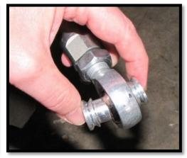
25. Connect the heim joint to the collar on the control arm. Side a **12mm flat washer** onto a **½"** x **2-3/4" bolt.** Insert it though the clamp collar and heim. Secure it with a **12mm flat washer** and **1/2" lock nut**. Torque the nut to 110lb-ft. Repeat to other side.
