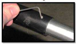
41. Located on each clamp collar are two **¼-20 x 3/8" set screws**. Make sure that the set screws are tighten so that the collars cannot move during use.
