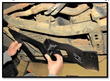
5. Slide a 1/2" flat washer onto (2) 1/2" x 1" bolts to connect the plate to the frame. Loosely secure them with 7/16" flat washers and 1/2" lock nuts.
