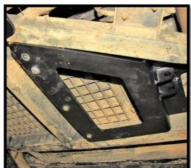
8. Install the driver side frame plate. Then Fasten all hardware and make sure that the plates are tightly secured.
