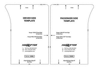
11. With the skid plate lying flat with the frame side down, place the templates down and follow the directions.
