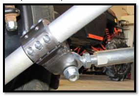
40. Located on each (hollow) bar is a single 1/4-28 x 3/16" set screw. Make sure that the set screw is tight so that the bars will not rotate during use. Do not over torque.
