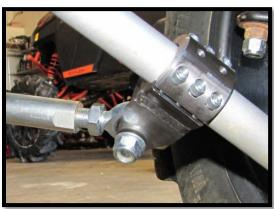
26. <u>Next, you must complete a CLEARANCE CHECK</u>. Follow the steps and check for clearance before riding. If you check before riding you can adjust before you damage the bars, clamps, or other parts.
