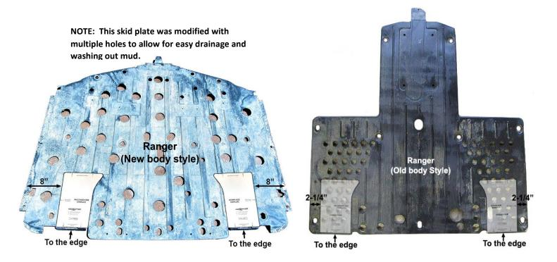
12. Cut the marked sections in the skid plate using an oscillating/cutting tool.
